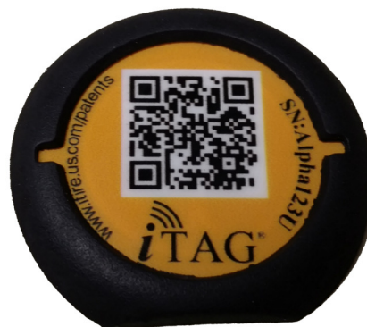
Figure 2: iTAG® in rubber carrier for tire application.
